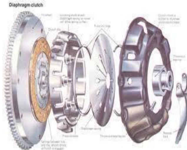
Fig: Diaphragm Spring Clutch
