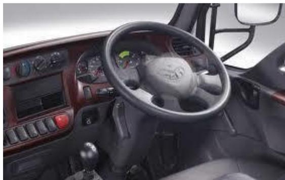
Fig: Tilt & Telescope Column
